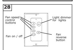
To control fan speed select from High, Medium or low speed buttons. To turn the fan off press the Fan on / off button. To dim lights press and hold button. To turn off light press and quickly release button. Press button marked REV to reverse the rotation direction of the fan blades
